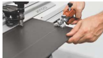
2. Cutting of Tile
